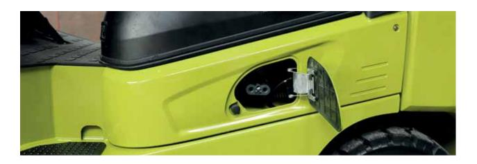
The Li-ion battery can be conveniently recharged via an opening flap on the side without having to open the battery cover.
