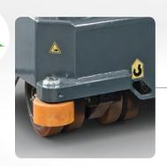
Fourfold load wheels for fast, intuitive multidirectional steering
