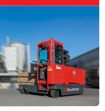
Our multidirectional sideloaders are equipped with up to two times of four-fold load wheels. which has the effect of low wear due to improved tyre rolling characteristics while steering.
